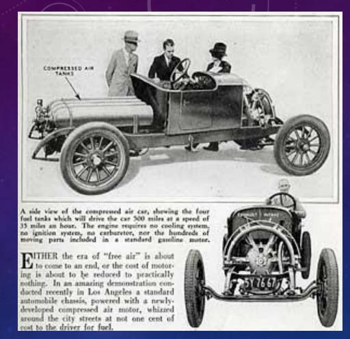
Compressed air car – 500 miles at 35 miles an hour with 4 compressed air cylinders
